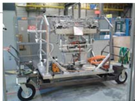
The LHC collimator prototype used for the test
